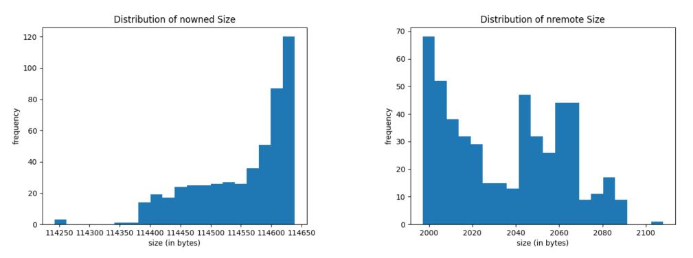
Distribution of nremote and nowned parameters from CLAMR utilizing using 288 processes across 8 nodes. The CLAMR job used a grid size of 5734 and ran for 500 timesteps.
